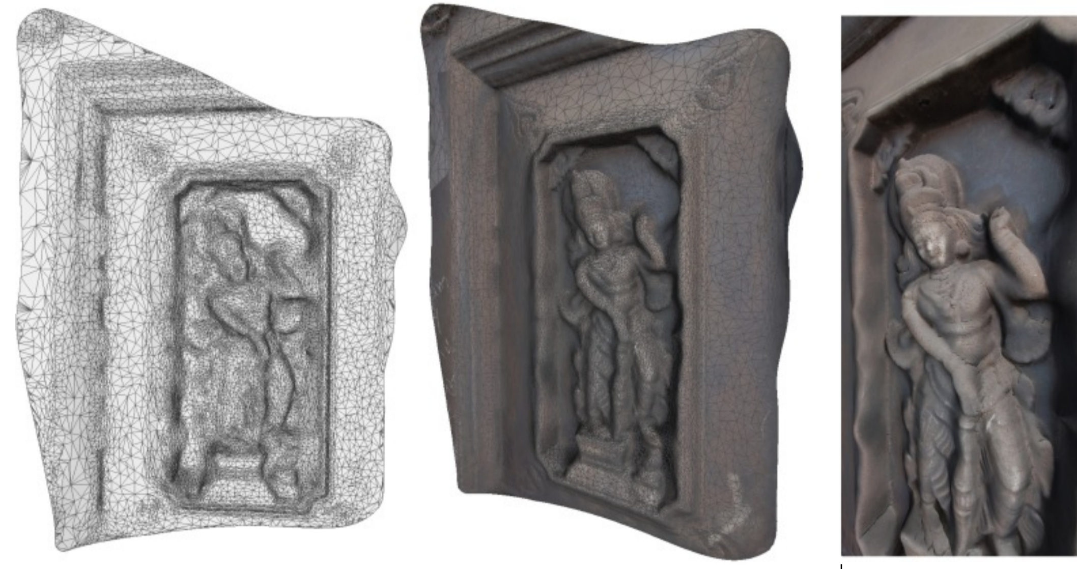
Figure 3: Reconstructed and textured mesh [8] from the four images in figure 2.
