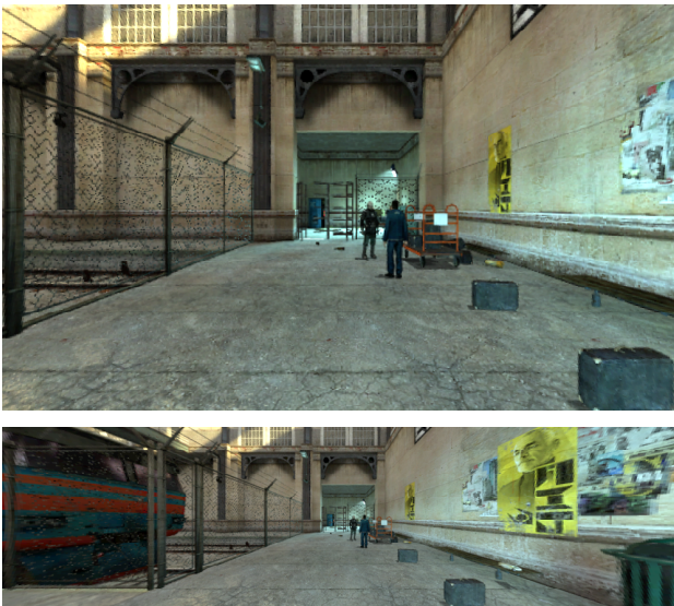
Figure 2. 100 degree (top) and 140 degree (lower) horizontal field of view using a perspective projection.
