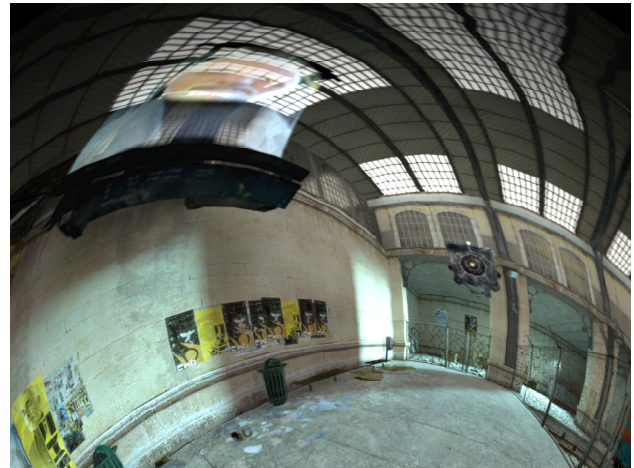
Figure 4. Example of a warped image for projection onto a hemispherical dome after reflection from a spherical mirror.
