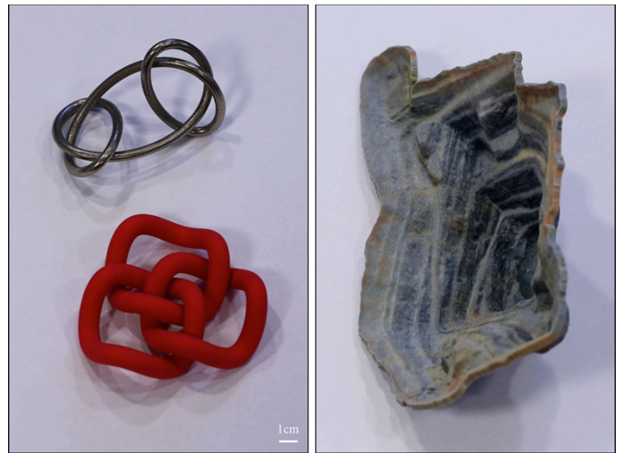
Figure 7. Mathematical knot illustrates circle extruded curves (left), extruded mine model surface (right).
