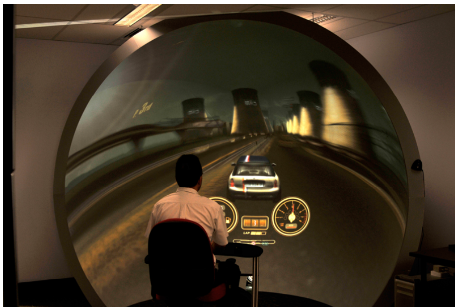
Figure 6: iDome and car racing game example. While the warped image sent to the data projector (figure 5) appears distorted, the imagery is perfectly correct on the dome surface.
