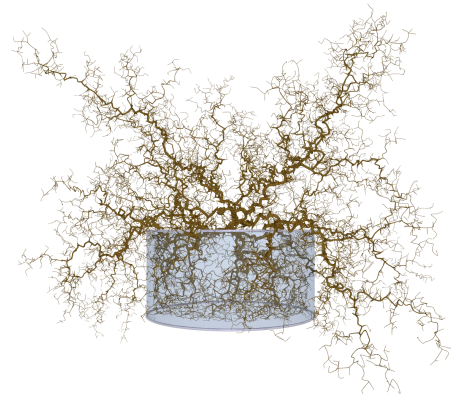
Figure 3: DLA constrained within an open can (a cylinder sealed at one end but open at the other end). Particles are added randomly on the surface of a sphere with the origin at the centre of the top face of the cylinder.
