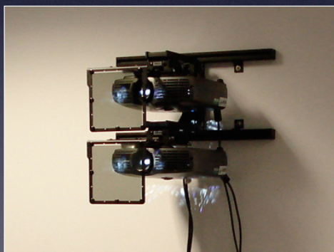
Twin projectors, one for each eye image
