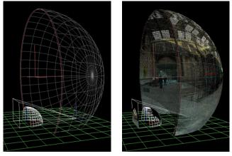
Figure 4. Example of ray casting simulation, model of physical geometry and projector specifications (left) and verification of simulated projection test (right).
