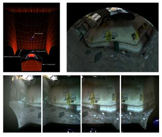
Figure 7. Optical simulation using raycasting into an accurate room model, top/left. Projected image that results in an undistorted view, top/right. Photographs of the actual room in 4 segments, note the camera is located further back from the ideal viewing position.
