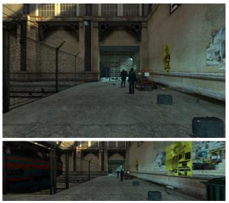
Figure 1. 100 degree (top) and 140 degree (lower) horizontal field of view using a perspective projection.
