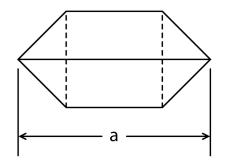
Figure 1. Side view of the ring dodecahedron. The lines trace its edges. The dashed lines show the hidden edges where the hole passes through it. The dimension a is the repeat period of the cubic unit cell.
