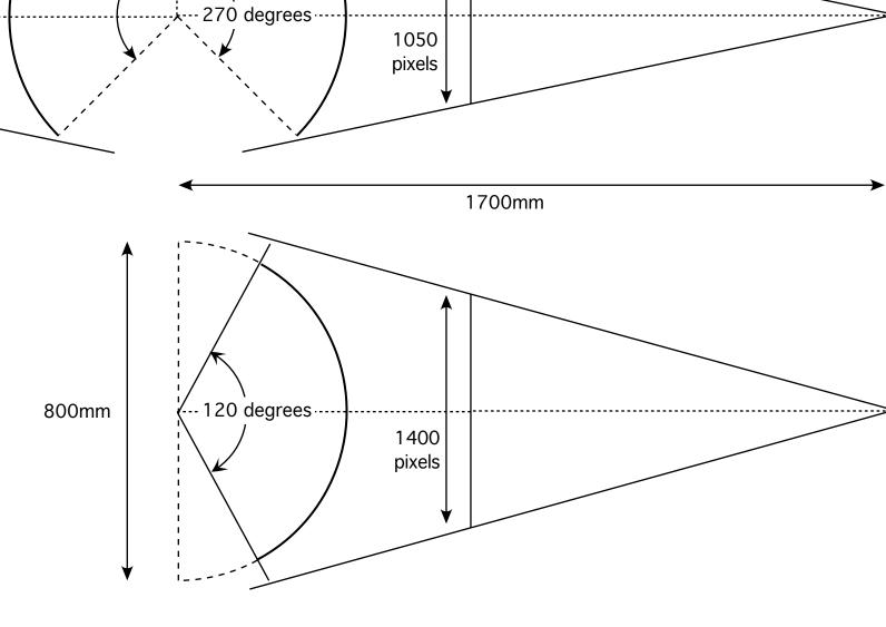
Content generation (for example Unity3D) is achieved by the rendering to texture of three prespective views (100x120 degree FOV). These three textures are then each applied to a mesh (one for each projector) that implements the geometry correction and edgeblending. This is a total of 3 x scene renders, 3 x texture passes.
