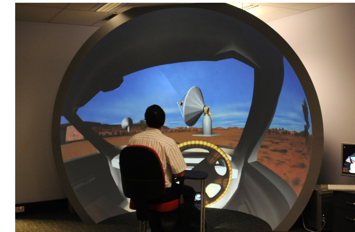
Figure 7. Driving simulator as part of the ASKAP (Australian Square Kilometer Array) site exploration "game". Developed with the Unity engine.
