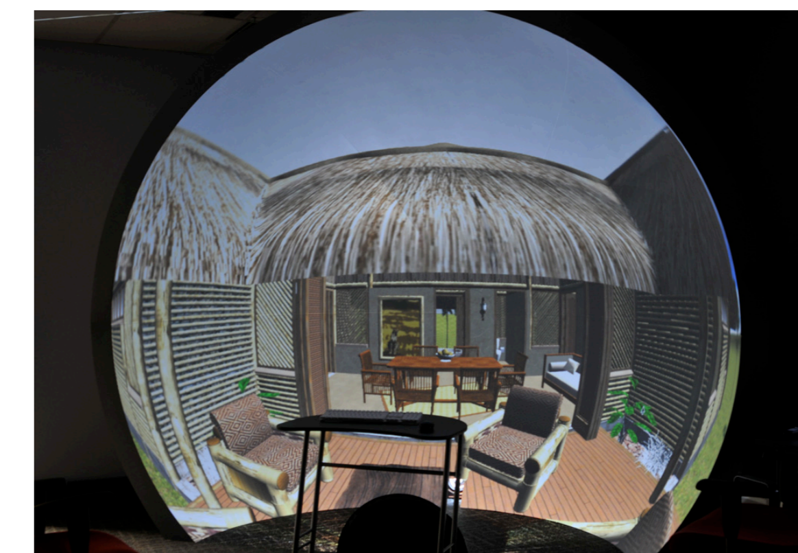
Figure 8. Example of architectural visualisation. Models created in Google Sketchup and converted into an environment developed with the Unity engine.
