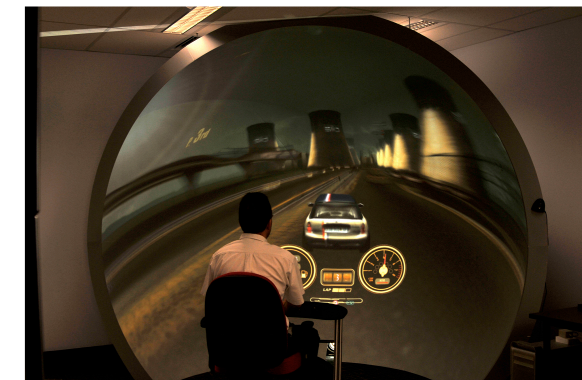
Figure 9. Car driving simulator used in the quantitative analysis of the effects of alcohol on driver performance. Developed with the Blender realtime engine.
