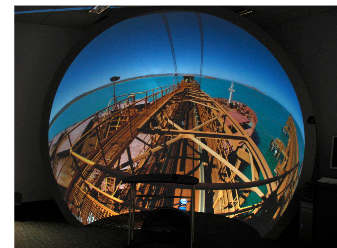
Figure 10: Remote operations using realtime footage captured with a 360 degree video camera, the LadyBug-3.
