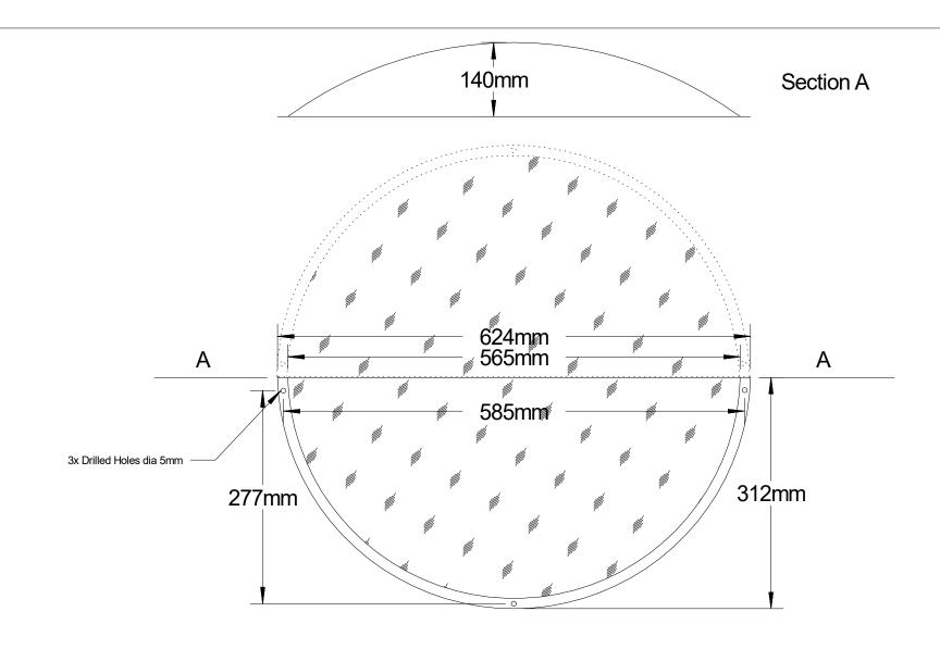
Material Thicknesss: 3mm
